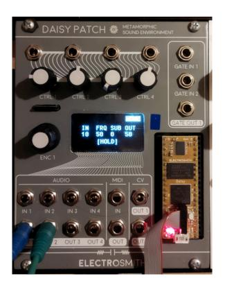
The module can be used simply by picking the audio output from the OUT1 output (OUT1/OUT2 if you want a stereo signal), no other connections are needed unless you want to add (or extract) some modulation. When you use the module for the first time set the knobs in this way:
